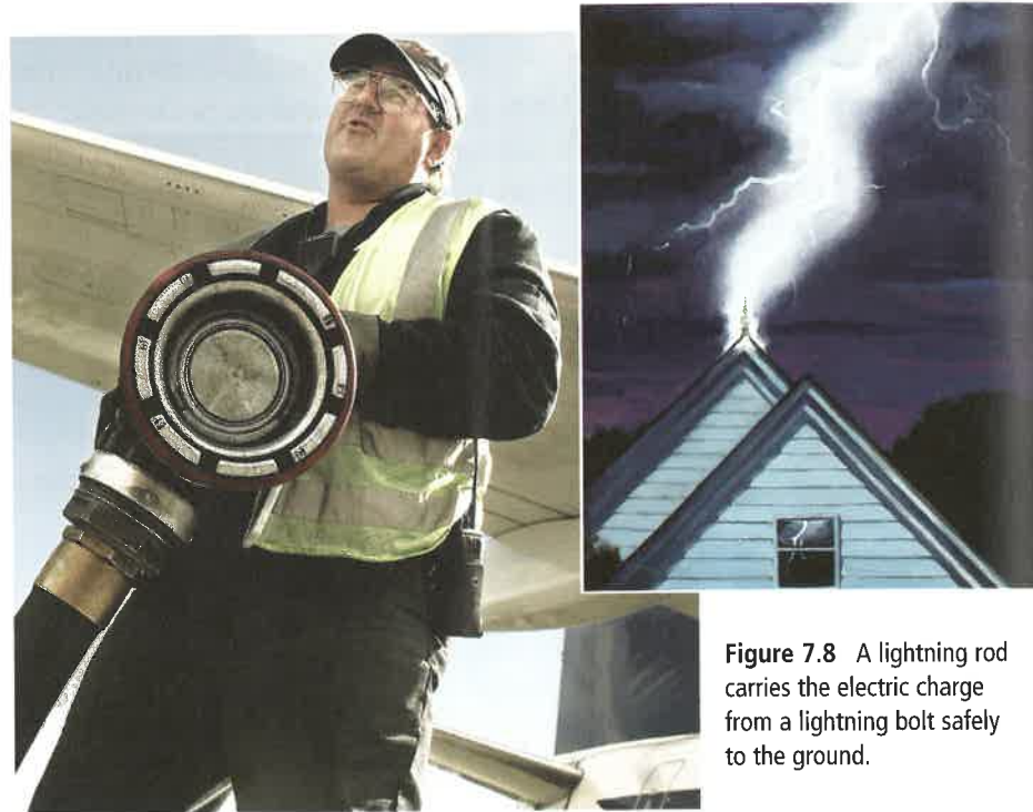
Figure 7.7 As a fuel truck drives down the highway or an airplane lands on a runway, it can become charged. The excess charge has no way of escaping because it cannot move through the rubber tires. A small spark near the fuel could cause a huge explosion. Therefore, the fuel hose includes a grounding cable to prevent sparking.
